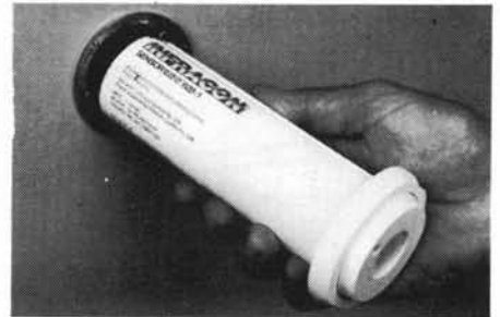
Above — Infracon sensor cylinder 2" in diameter being inserted into ceiling.
