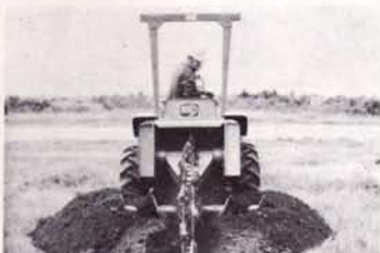
Double-auger digging assembly.
