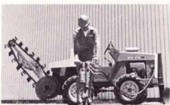
Hydraulic pavement breaker.
