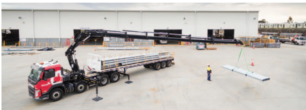
The HIAB XS 288 E8 HiDuo crane is mounted on a Volvo FM 8x4 with a 13.5m trailer
