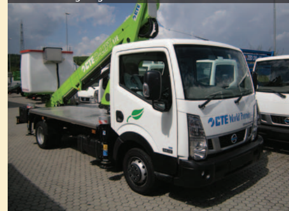
The CTE B-LIFT 17E from CTE Aerial Platforms has 16.6m working height
