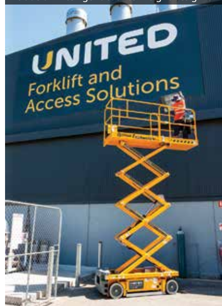
Optimum 8 electric scissor lift safety features include an intelligent counterweight design
