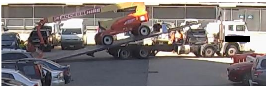
Image 2: Depicts the machine commencing its uncontrolled movement down the raised tilt tray truck platform.
