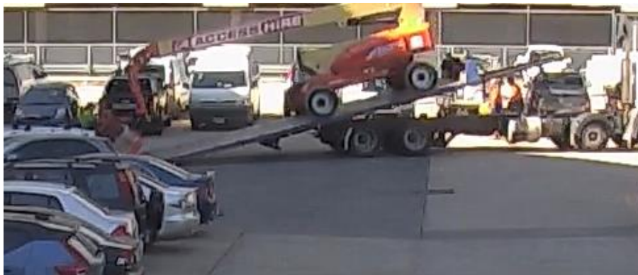
Image 1: Depicts the point of contact between the tray and the basket with brake wheels slightly raised off the truck tray.
