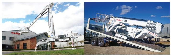
The 3315 Spider Lift from Monitor Lifts is a dual telescopic knuckle boom which allows 17m of up-and-over reach
