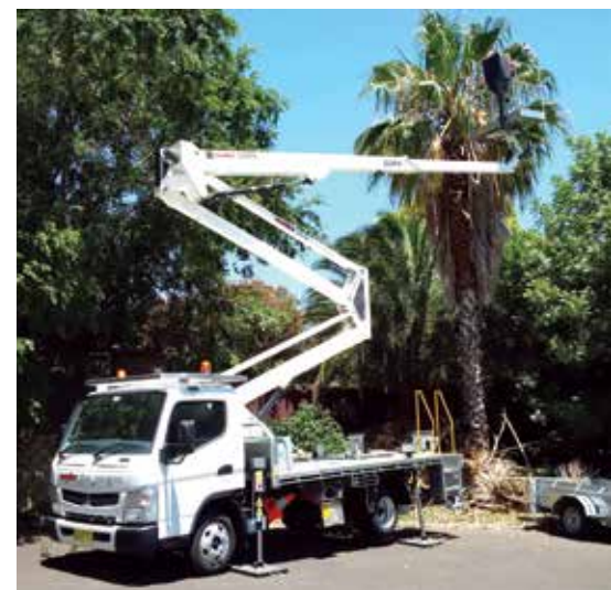
Monitor Lift's E209PX is a compact 20m truck mounted EWP that can be driven on a car licence
