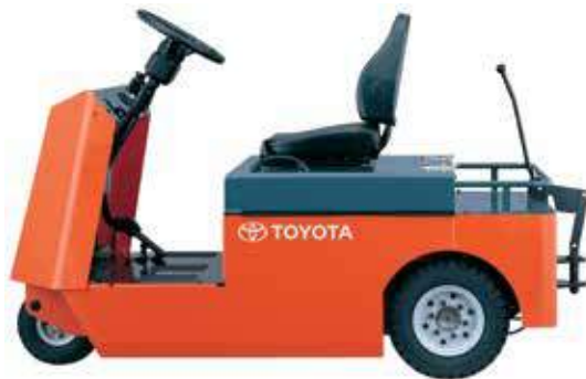
Two new electric-powered Toyota CTB6 sit-down type towing tractors now carry for Wideline reducing manual handling
