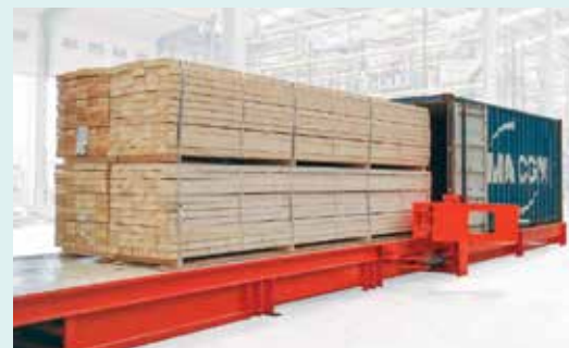
The new container slip-sheet loading system can load a container in as little as six minutes
