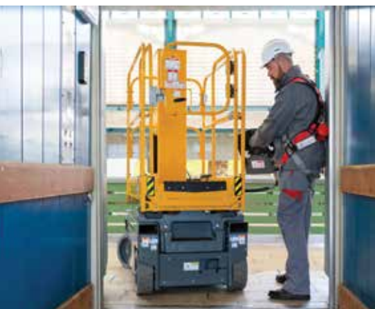
The Star 8S has a load capacity of up to 230kgs and the ability to work efficiently and confidently up to 8m
