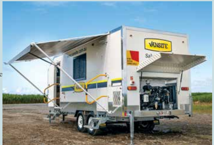
Vansite vans are an all in one site application and have everything needed in one unit - generator, kitchen, office, light tower etc
